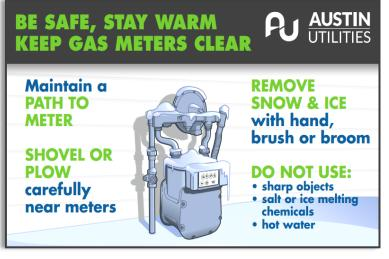
make sure ice has not accumulated on the gutter above the meter. If you have accumulated snow or ice on your meter, take proper care to remove the snow or ice carefully with a broom or brush. Never kick or hit your gas meter or its piping with a shovel, hammer or any hard object to break away built-up snow or ice.
